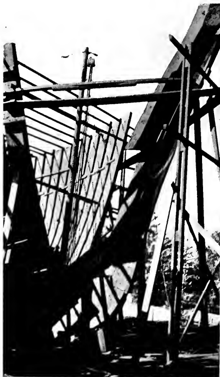
Bow framing of a big auxiliary schooner.
